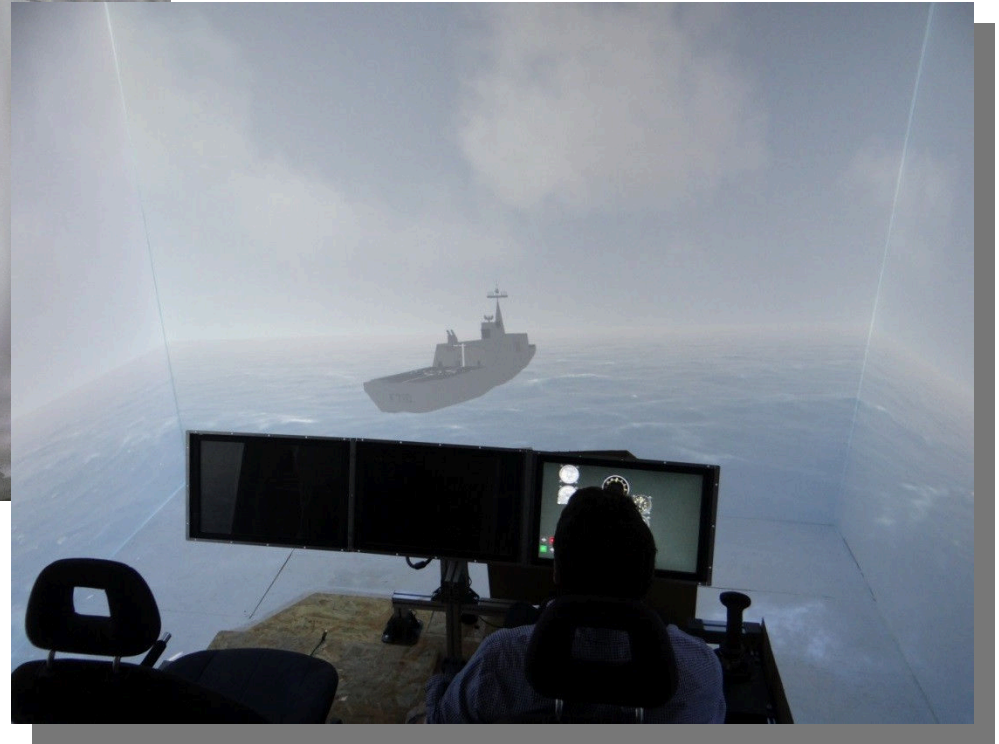
Four faced cuboidal CAVE simulator
